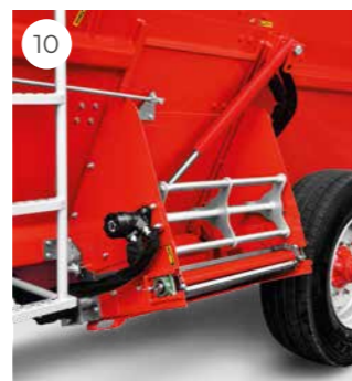
10 Fixed unloading conveyor with rotary magnet
