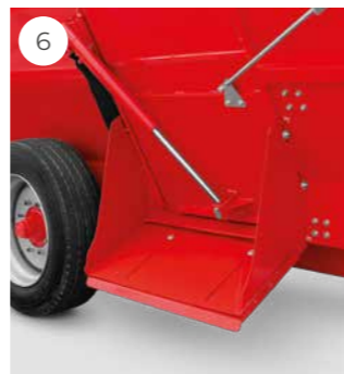
6 Direct discharge by chute
