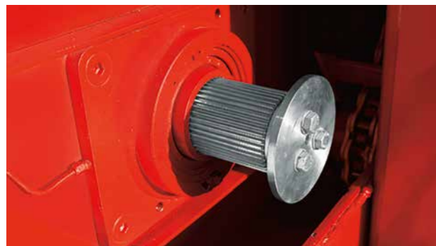
B SPLINED PROFILE SHAFTS for a uniform power transmission and a quick maintenance.
